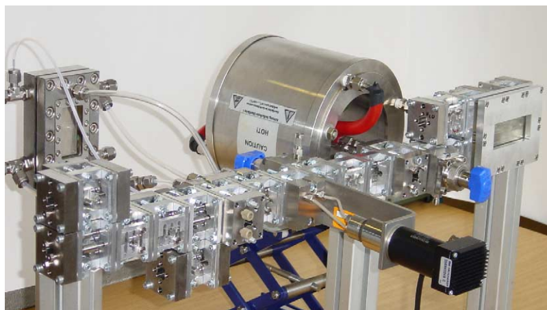
Fig. 16. Microplant used for the sulfonation of toluene.
