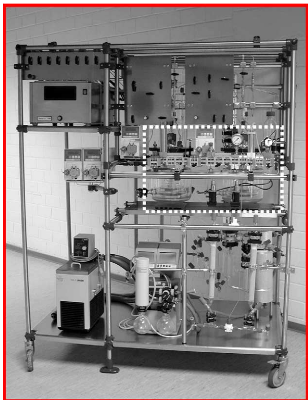
Fig. 5. Laboratory-scale miniplant with microplant (within hatched line).
